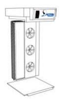
The cell/tunnel has one lane with an evaporation unit, which is supplied by a refrigeration unit/cooling plant. An evaporator/ventilator unit consists of a coil positioned on the side of a central ventilation column (see schematic diagram opposite).
