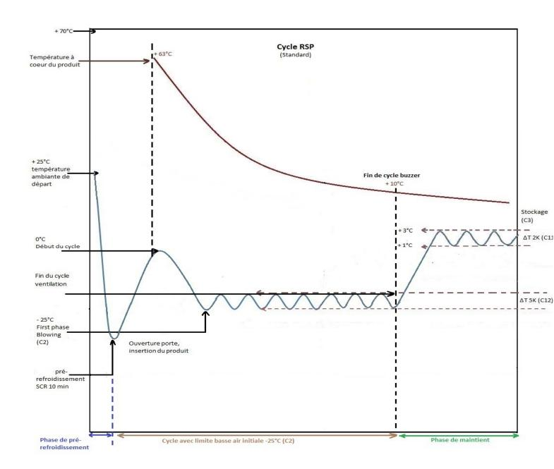
2.2. Sequenced cycles (typical diagram, use and setting via parameters, see manual)
