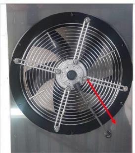
✓ Attaching the evaporation/ventilation units:
